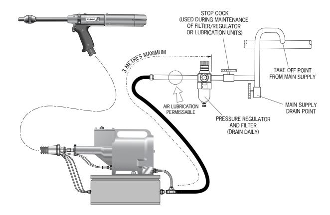
Follow the steps below when connecting the tool to the intensifier and main air supply:
